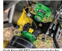
Quik Knect™ PTO receivers make for easy PTO connections in seconds.
